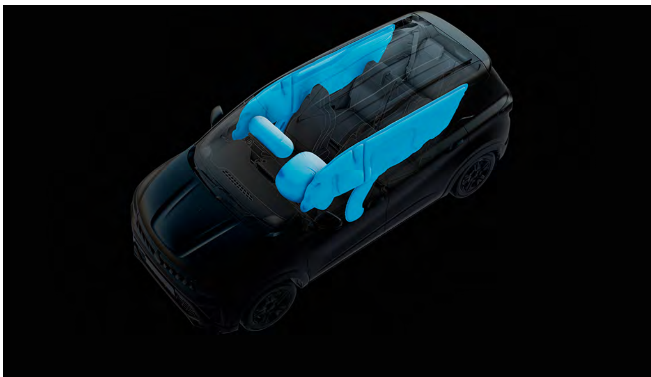
6 airbags Six airbags offer increased protection.
